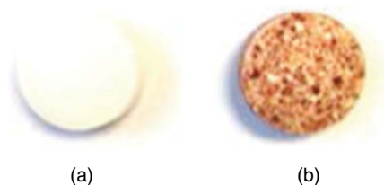
Figure 1.3 (a) Initial and (b) aged tablets containing drug substance sensitive to local pH environment provided by a minor excipient (<10 wt%). The aged tablet was exposed to 40 °C and 40% RH for 2 weeks.
